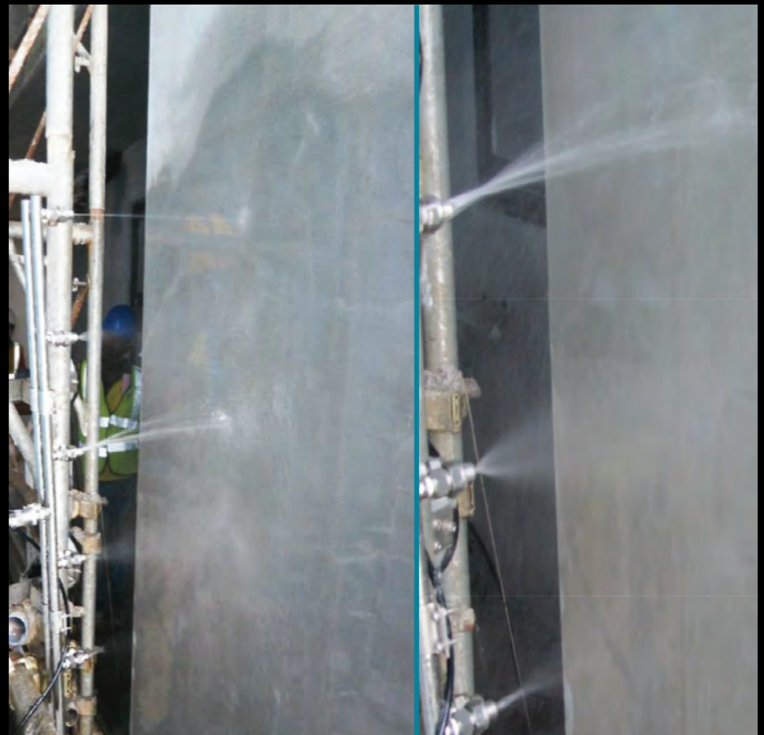
WATER TIGHTNESS TEST = 0% SEEPAGE
