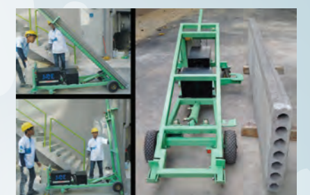
JOE PIM PANEL INSTALLATION MACHINE
