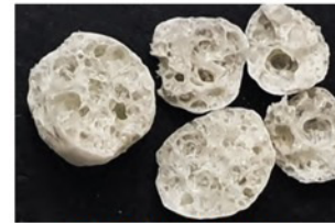
Non-Structural LiGrA Loosely packed coarser pores
