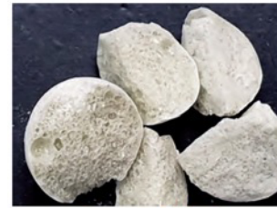
Structural LiGrA Densely packed finer pores
