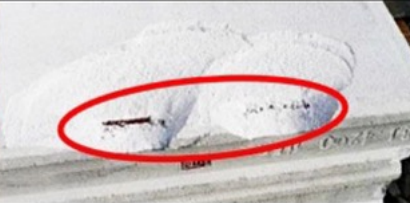
Porous, Corrodes BRC inside, Bending and No Strength
